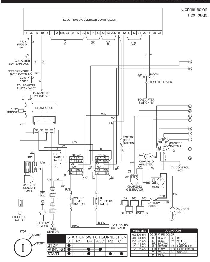
Figure 83. Engine Wiring Diagram
